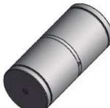
Pino Traseiro Comp. Total: 168,00mm Diâmetro: 80,00mm
